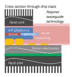
Athermalisation is demonstrated by intimate short-loop control and on-chip temperature monitoring. The use of InGaAlAs active layers enables the gain elements to operate at the required higher temperatures.
