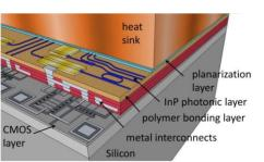
A schematic of the combined photronic IC's stack is shown in the figure.
