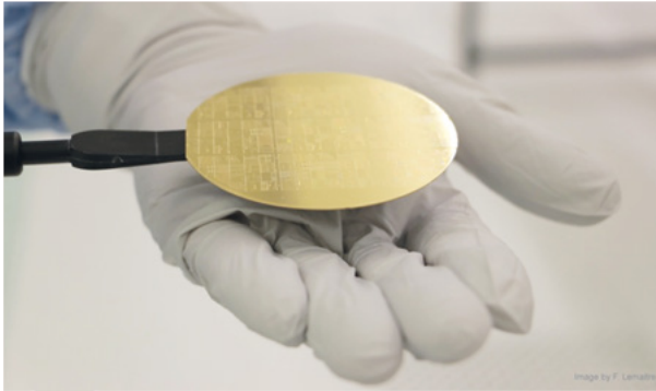
Figure 1 3" wafer fabricated on the InP generic technology platform of SMART Photonics. Image by F. Lemaître.
